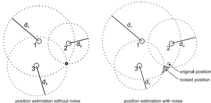
**Figure 1.** Influence of measurement error on quality of node's estimated location
