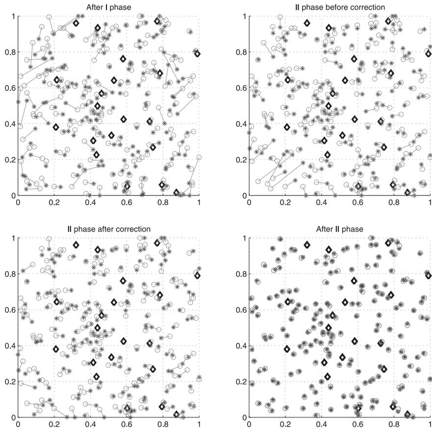
**Figure 4.** Simulated annealing in network nodes localization
