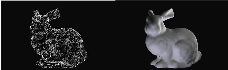
**Figure 1.** Reconstruction problem. On the left – a set of 3-D points P, on the right - surface S.
